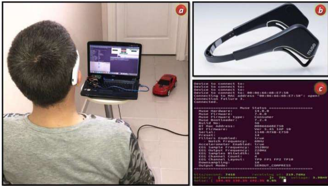
Figure 5 a) Prototype of the developed model b) EEG device used in this study c) software development interface
