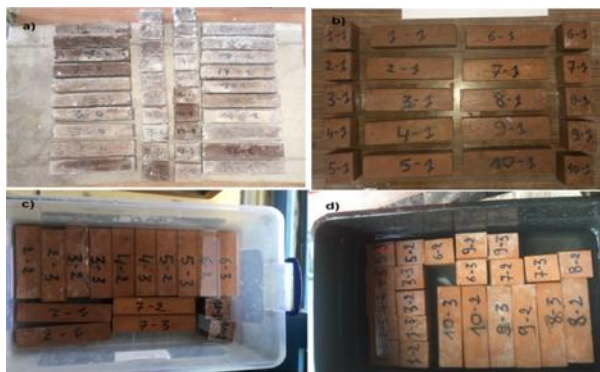
Fig.1. a) Samples after exposed to ( \text{MgSO}_4 ), b) Samples after exposed to ( \text{Na}_2\text{SO}_4 ) c) Samples while exposed to ( \text{MgSO}_4 ), d) Samples while exposed to ( \text{Na}_2\text{SO}_4 )
