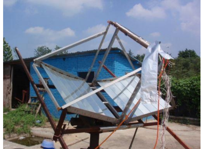
Figure 3. Experimental set-up of water-cooled CPV module [23].
