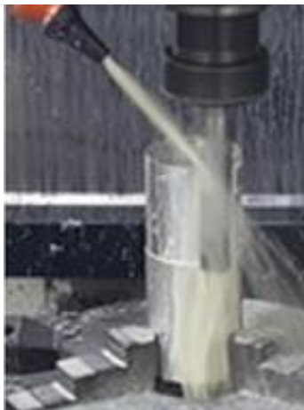
Figure 1. CNC milling operation of aluminum and steel pipe
