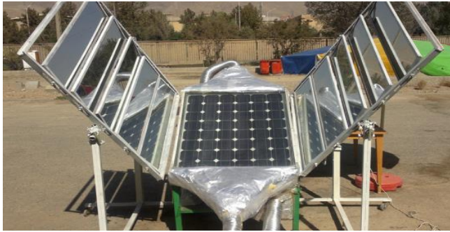
Figure 17. The PV/T collector and Fresnel reflector [56].
