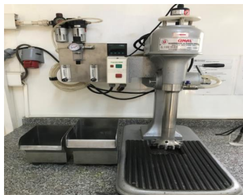
Figure 2. The flotation device used in the experiments.
