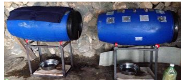
Fig 2. Barrel A with odor control cover (left) and Barrel B without cover (right)
