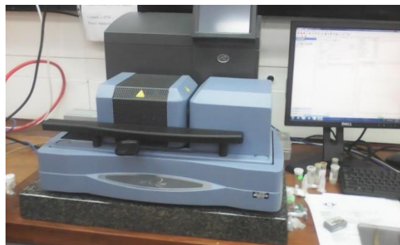
Figure 1. Photograph of TGA Q50 thermogravimetric analyzer used.
