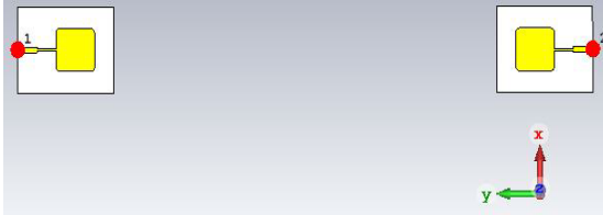
Figure 11. Two identical antennas placed in the far field region of each other for group delay analysis
