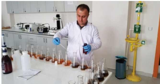
FotoĖraf 13.   zeltiye difenilamin indikat  r  eklenmesi. Photo 13. Adding diphenylamine indicator into solution.
