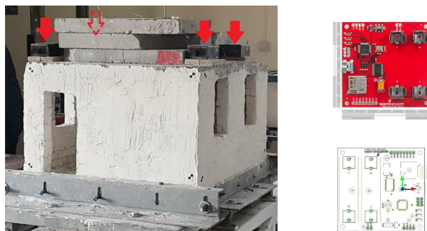
Figure 8. Location points of accelerometers and the ADXL 345 accelerometer
