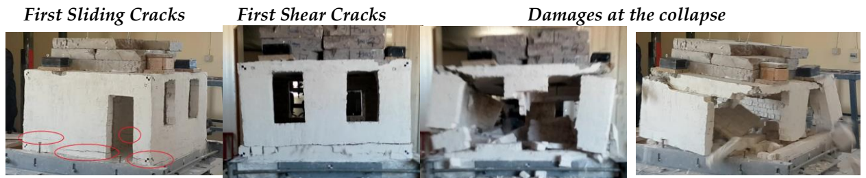
Figure 14. Cracks and damage were observed at the Specimen 1
