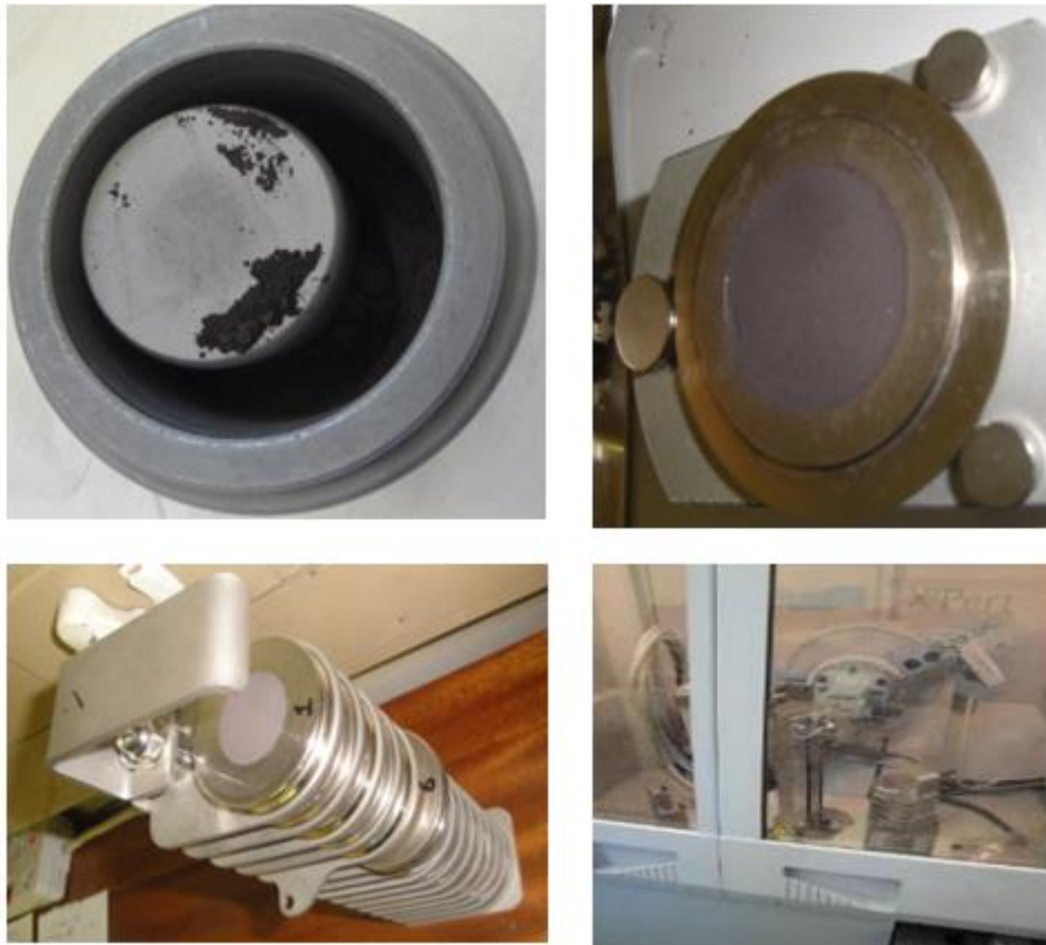
Figure 4 Sinter sample preparation of X-ray diffraction analysis.
