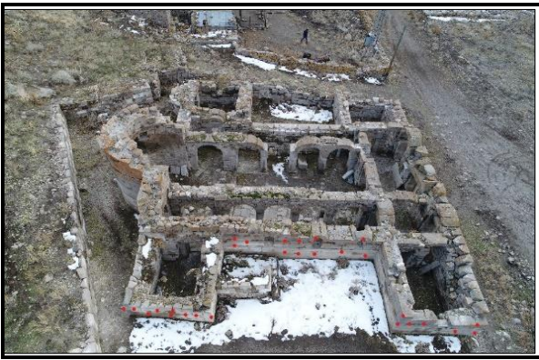
Figure 4. The building control points and the distribution of control points of the side facade of the building
