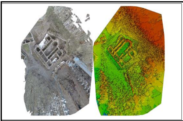
Figure 7. Orthophoto and digital surface model (DEM-DSM) of the study area
