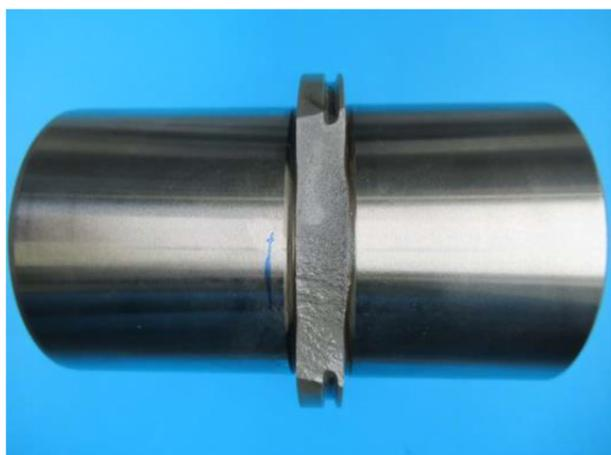
**Figure 1.** Images of the (a)original, and (b)broken kingpin part
