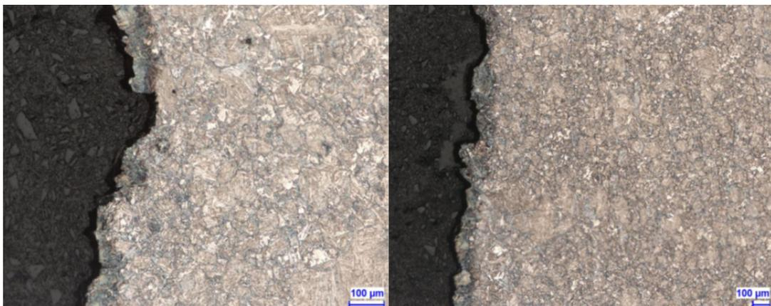
Figure 5. Images of the FR sample showing a mixed structure of bainite and coarse martensite phases
