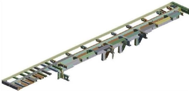
Figure 2. Demountable trailer chassis analysis model (half)
