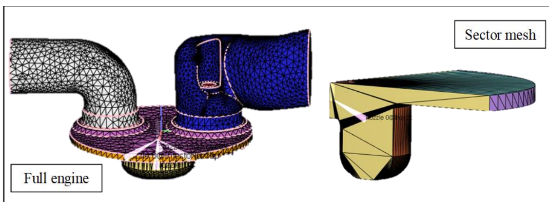
Figure 3. The fluid domain of the CFD model as a sector and full engine at TDC.
