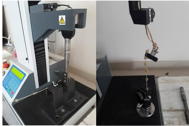
Figure 3. Stalk cutting and flower rupture tests.
