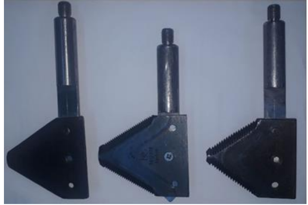
Figure 2. Types of knives used in cutting tests (smooth, fine toothed, coarse toothed).
