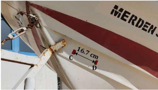
Fig. 5. User tie points and scale constrains – 2
