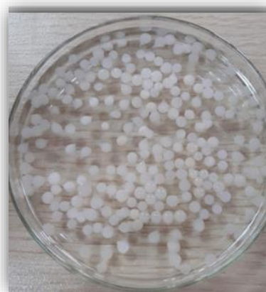
Figure 2. The preparation of immobilized beads
