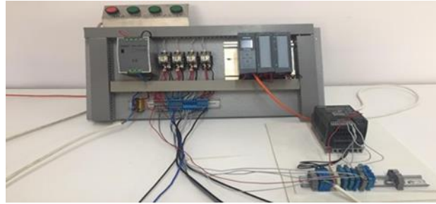
Figure 5. Siemens Sinamix V20 asynchronous motor drive with S7-1500 PLC connected in laboratory environment
