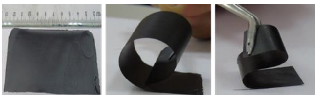
Figure 4. The bending and surface photographs of GO-3 film obtained by casting
