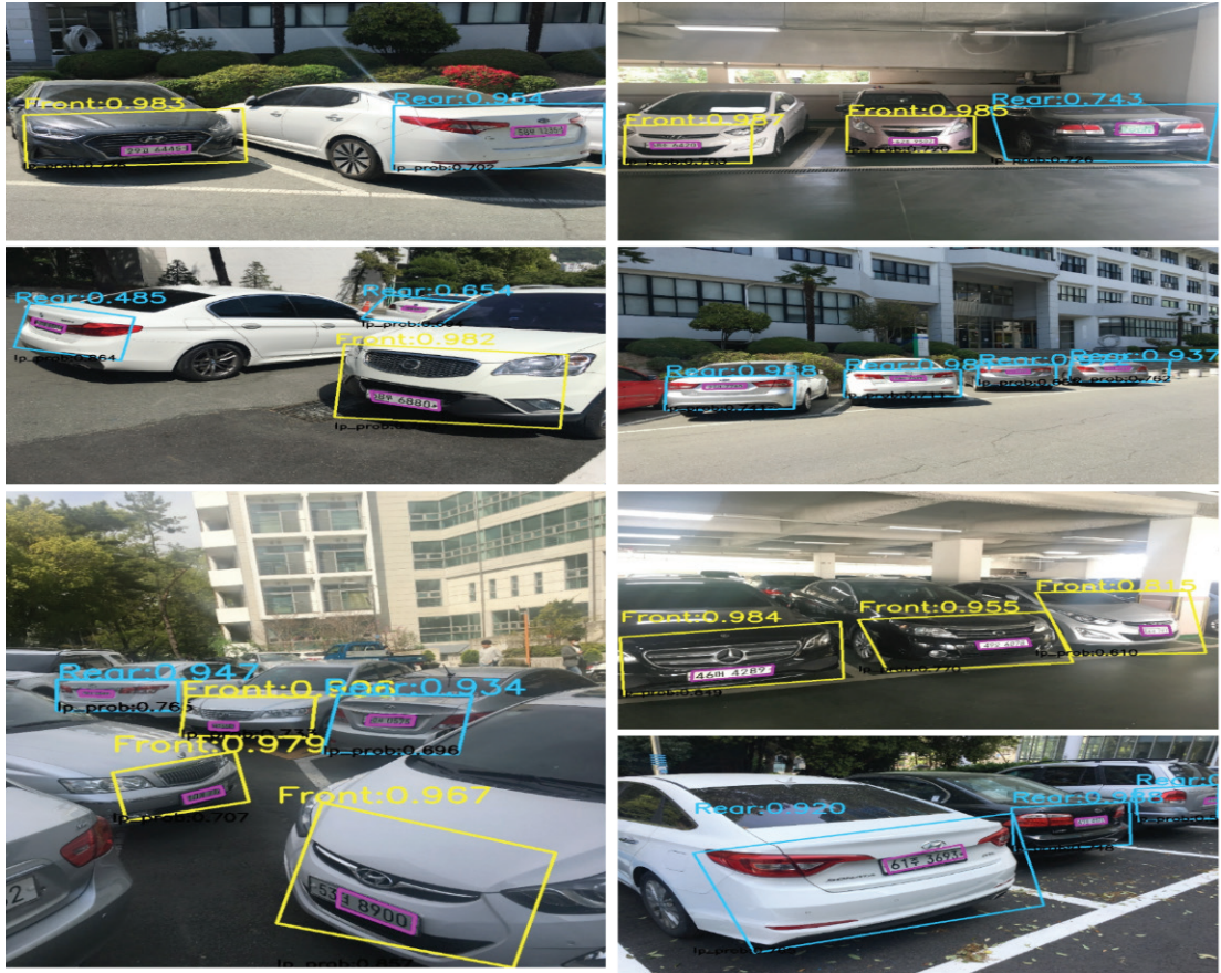
Figure 10. Classification and pose estimation results of Multiple Cars Scene dataset
