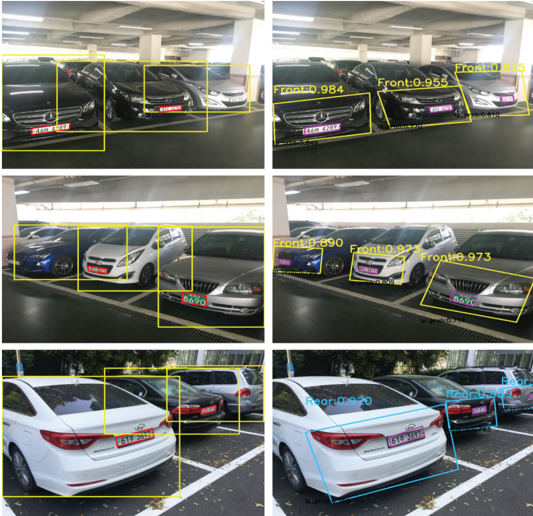
Figure 11. Comparison between vehicle pose estimation and license plate localization (left column) and proposed method (right column). On the left side, pose estimation and license plate localization missing appeared due to the false regression of license plate; on the other hand, our proposed method can avoid those cases and find all of the license plates
