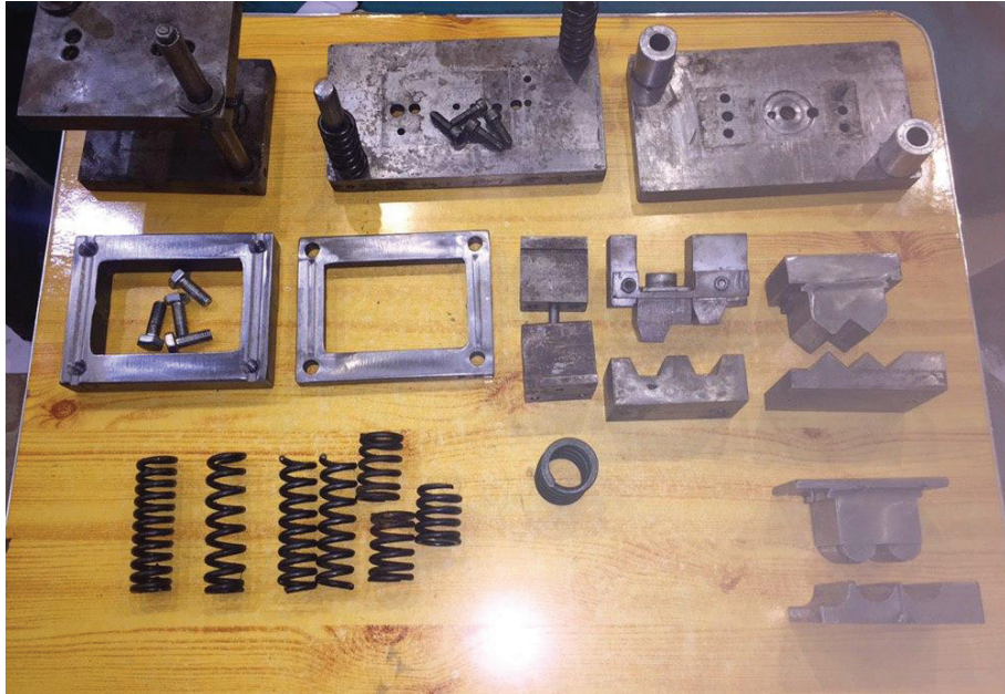
Figure 2. Three dies with double circular, rectangular, and triangular profile with and without drawbead with their accessories
