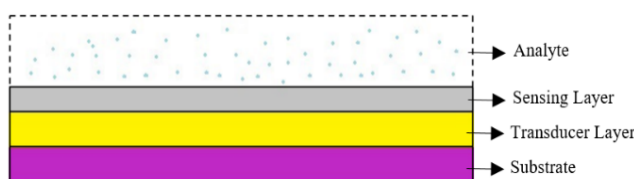
Figure 1. MEMS-based gas sensors layer structure
