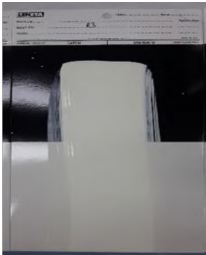
Figure 5. Hiding test result for optimum experiment (No: 4)
