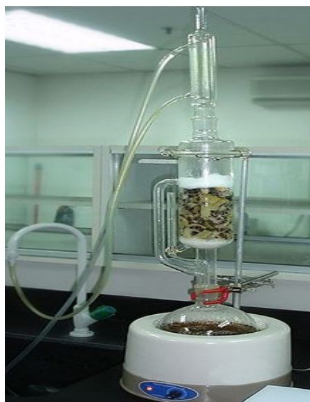
Figure 1. A schematic representation of a Soxhlet extractor
