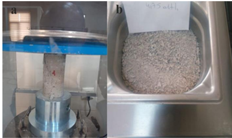
Figure 2. Experimental studies (Sample prepared for uniaxial pressure experiment and \text{Na}_2\text{SO}_4 experiment)
