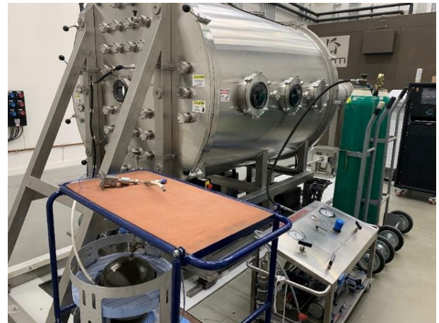
Figure 4. Thrust chamber test setup
