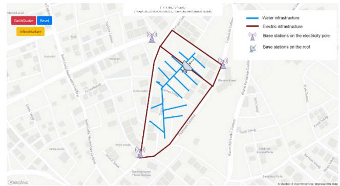
Fig. 6: Post-Disaster Prototype Interface for Infrastructures
