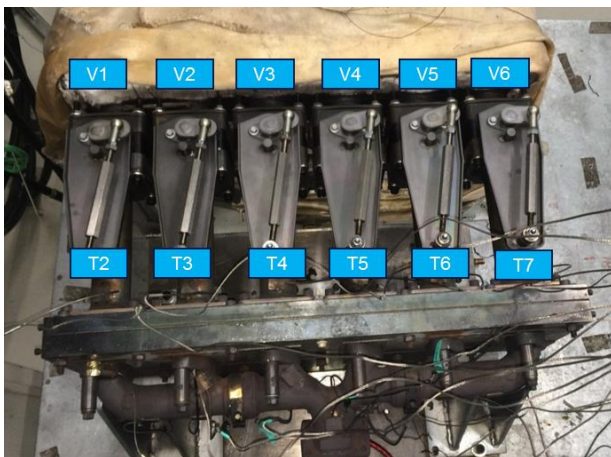
Figure 17. Exhaust manifold test rig with EGR valves
