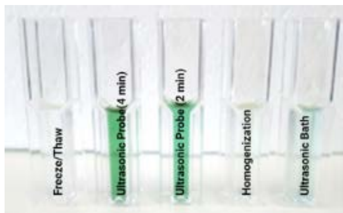
Figure 2. The supernatant of frozen biomass collected after performing cell disruption by freeze/thaw, ultrasonic probe, homogenization, and ultrasonic bath methods.
