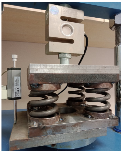
Figure 3. Compression test of the spring plate
