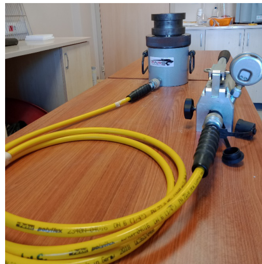
Figure 4. The pull-out test equipment in this study
