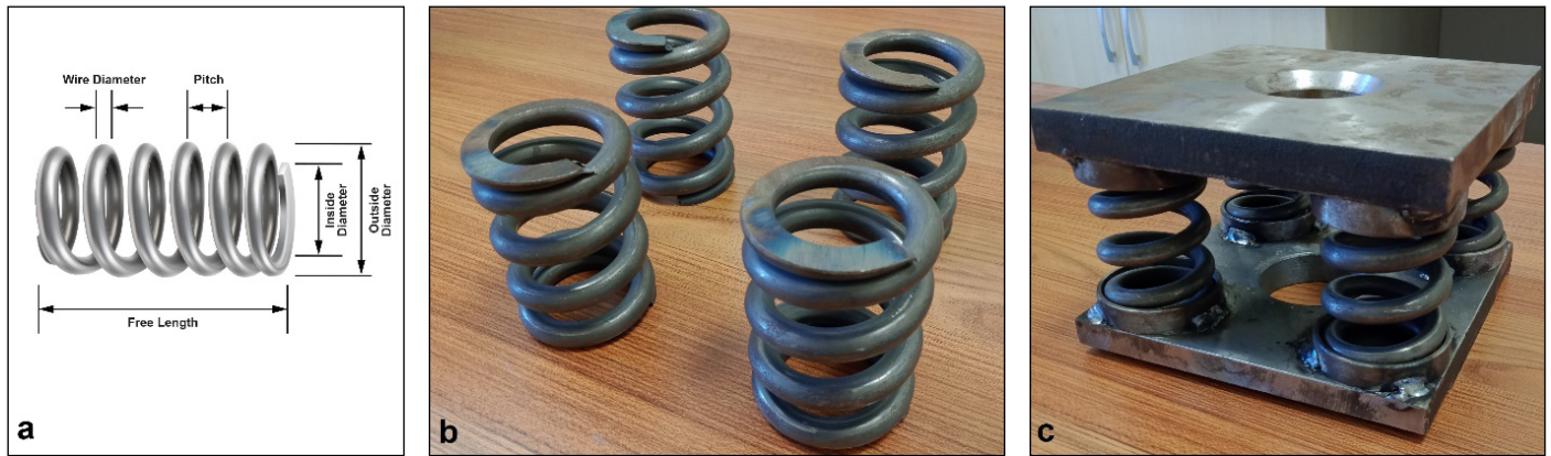
Figure 2. Size parameters of springs (a), springs (b) and the spring plate (c) used in this study
