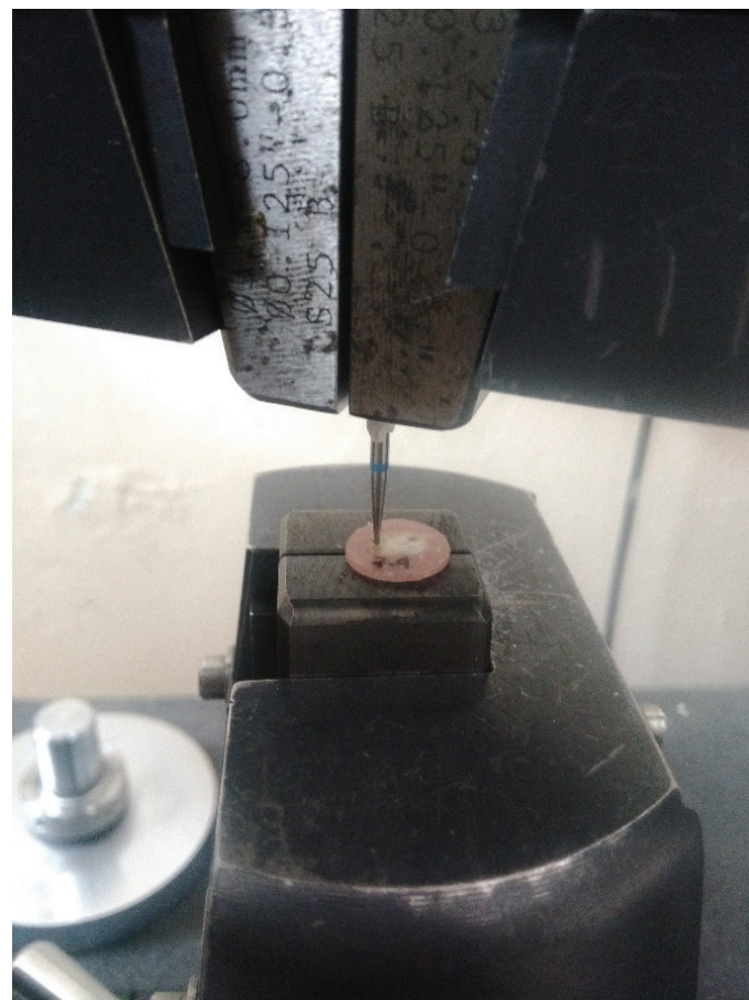
Figure 3. Loading was performed on a universal testing machine at 0.5 mm/min speed until material dislocation occurred.
