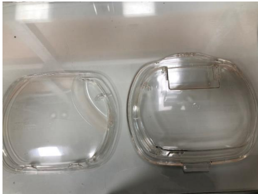
Figure 1. Water tank upper and lower covers
