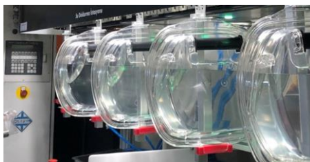
Figure 10. Automated leak testing system
