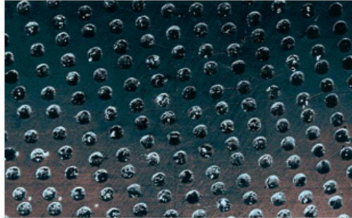
Figure 13. LST regular micro-surface structure in the form of micro-dimples [28]
