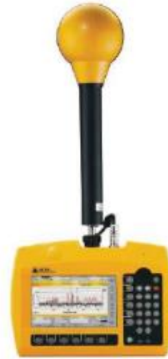
Figure 1. SRM-3006 device and triaxial antenna.
