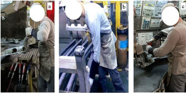
Figure 6. Arc welding line. (a) putting the part to the pallet repairs, (b) pallet push, (c) arc welding.
