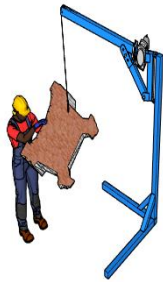
Figure 7. Part placement to the pallet with the manipulator.
