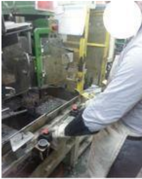
Figure 9. Automatic countersinking machine.
