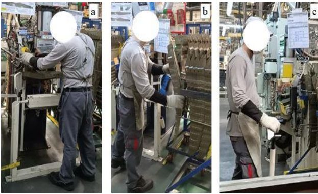
Figure 2. Manual welding line. (a) manual welding in the fixed spot machine, (b) part handling in Intermediate processes, (c) part hanging trolley pushing.
