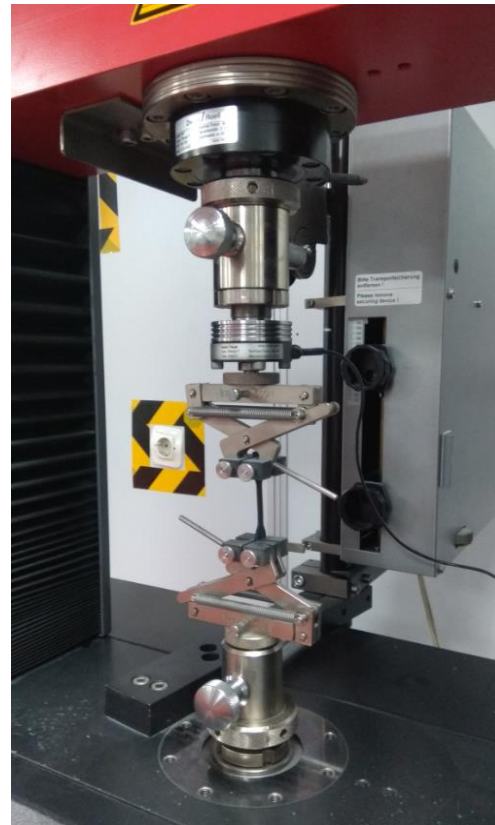
Figure. 1c. Tensile test device photo, sample, extensometer and force measuring device
