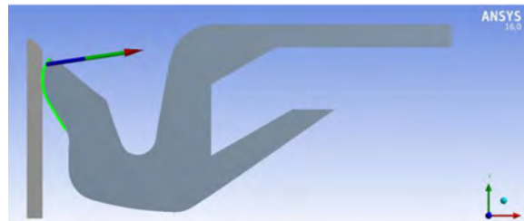
Figure 28. Total contact reaction force in 200 \mu\text{m} cover strictness (45,105 and 160 \mu\text{m} cover strictness is not shown, since they are same as 200 \mu\text{m} )
