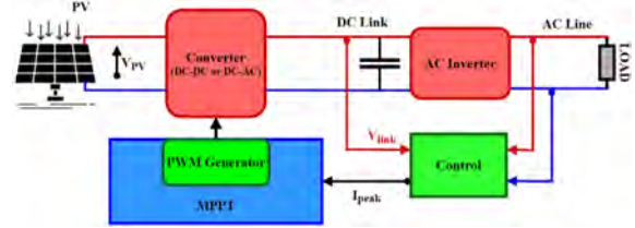
Figure 15. DC-Link capacitor scheme
