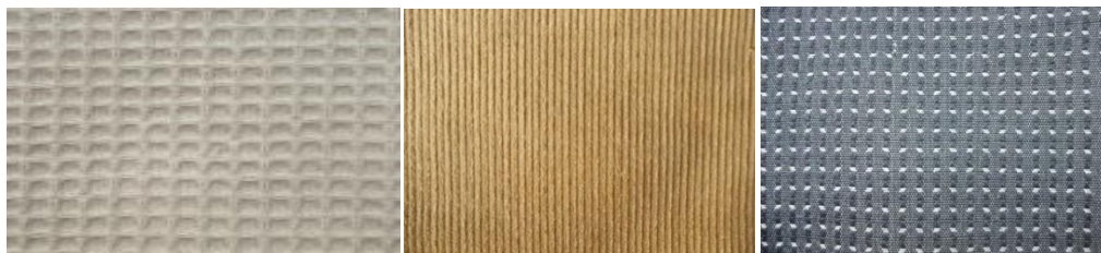
Figure 3. Samples No. 1.1, 1.2 and 2.2 with surface texture with increased friction against the air flow
