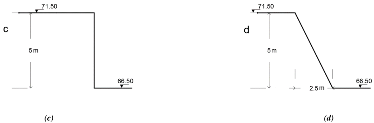
Figure 7. c and d sections with maximum elevation to be formed during 2nd basement excavation.
