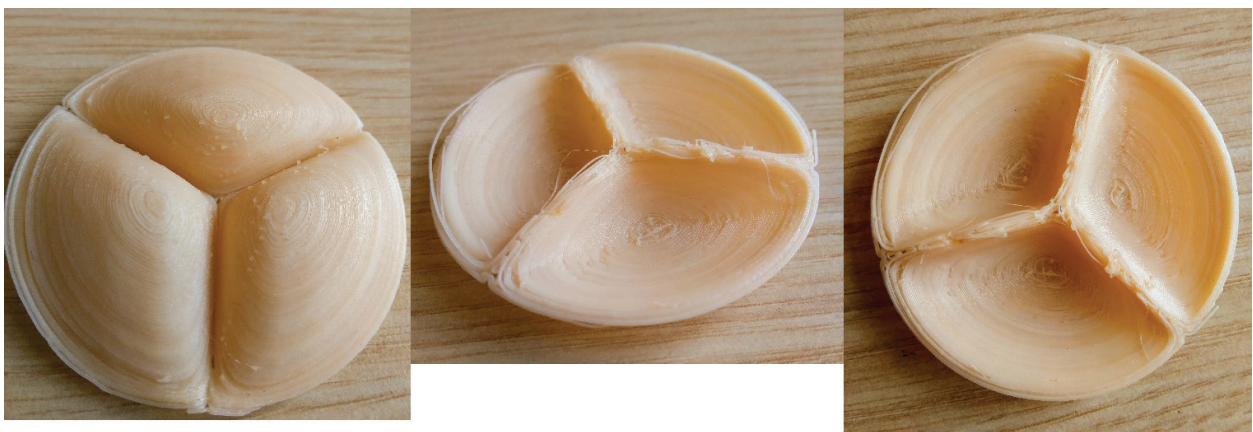
Figure 4: 3-D printing of aortic valve model made of soft filament
