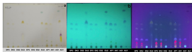
Figure 6. TLC chromatogram-5 visualized (a) under white light; (b) at 254 nm; (c) at 366 nm. Mobile phase: chloroform-toluene (75:25); derivatization: Vanillin-sulfuric acid reagent.
