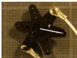
a) Servo horn used for finger movement of the InMoov humanoid robot arm [15]
