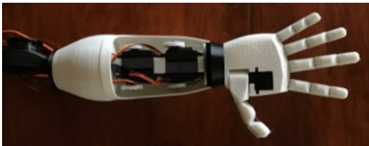
a) Arm design consisting of 4 servo motors used for the movement of the fingers in the original design
