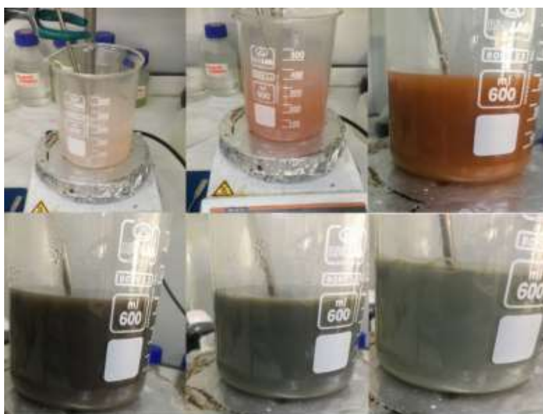
Figure 1. Color change with increasing temperature in AgNW synthesis
