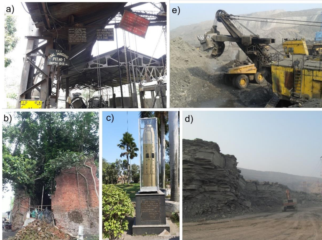
Figure 3: Photographs of the potential mining tourism sites, Raniganj Coalfield. (a) Mine cage and the signboard at Chinakuri pit. b) Old haulage room at Narankuri. c) Rescue capsule used in 1989 at Mahabir colliery. d) Excavated coal seam at Sonapur-Bazari OCP. e) Dragline-dumper combined operation at Khottadihi OCP.) Source: Photographed by the author.
