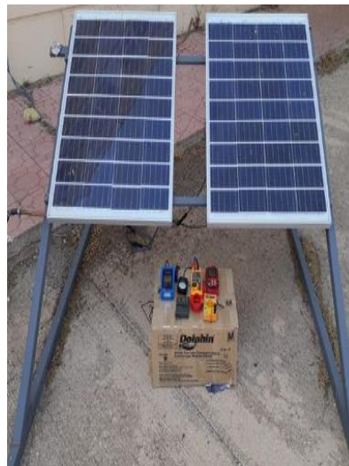
Figure 11. Measurement of solar panel temperature and other parameters
