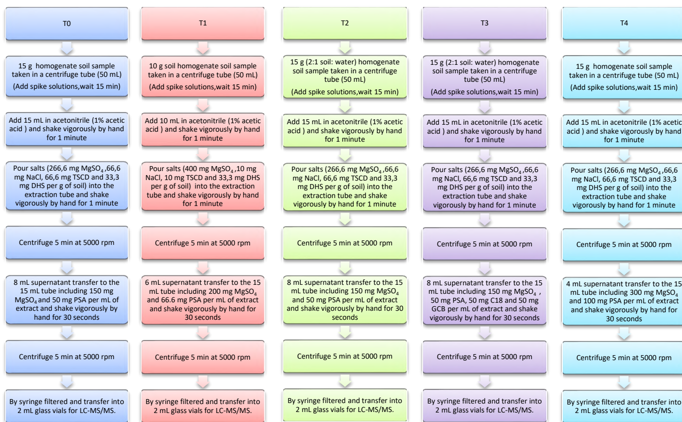
Figure 1. Analytical steps of modified QuEChERS for the analysis of chlorsulfuron and pendimethalin in soil samples
