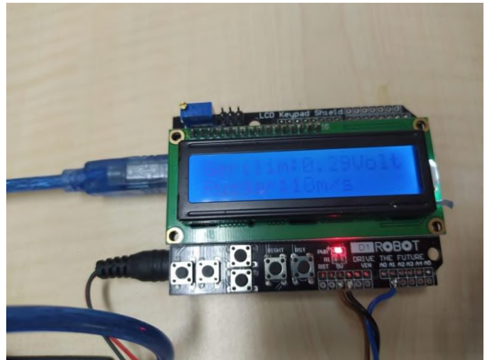
Figure 3. Display of wind speed and generated voltage on the LCD screen
