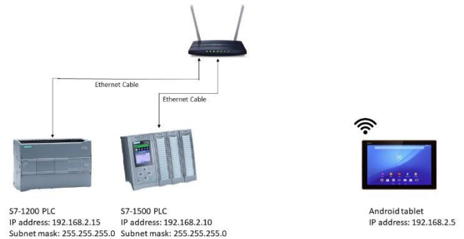
Figure 1.1: Topology of the system
