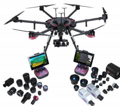
Figure 1. Some sensors used in UAVs for remote sensing
