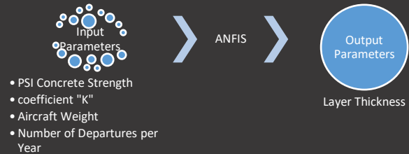
Figure 3. The main structure of the Fuzzy Logic model
