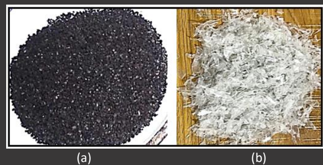
Figure.2. Materials used in this study, (a) crumb rubber (b) shredded plastic water cup.
