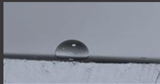
Figure 7. Position of the water drop on the bituminous mixture.
