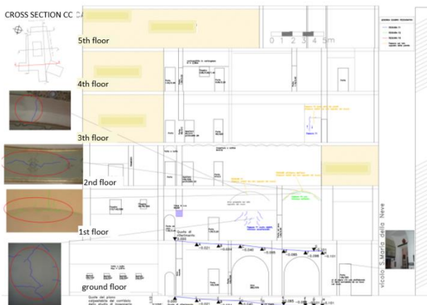
Figure 20. Crack map on the vertical wall in transversal cross-section C-C
