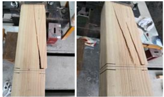
Figure 9. Midspan failure of S2 group
