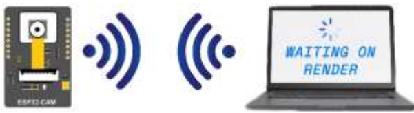
Figure 5. ESP32-CAM and local server communication.
