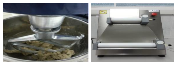
Fig. 1 Dough mixer and thinning machine
