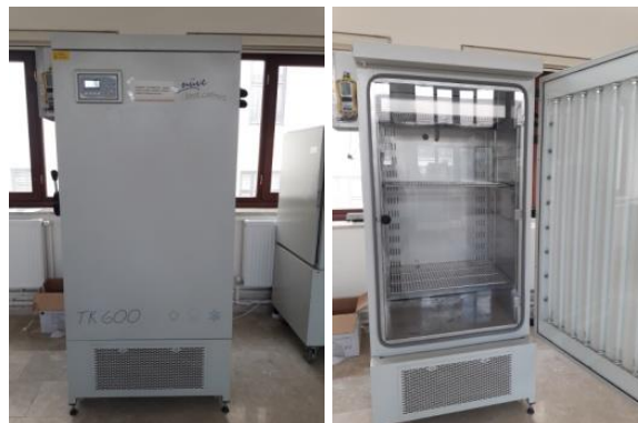
Figure 2. Climatic Test Cabinet
