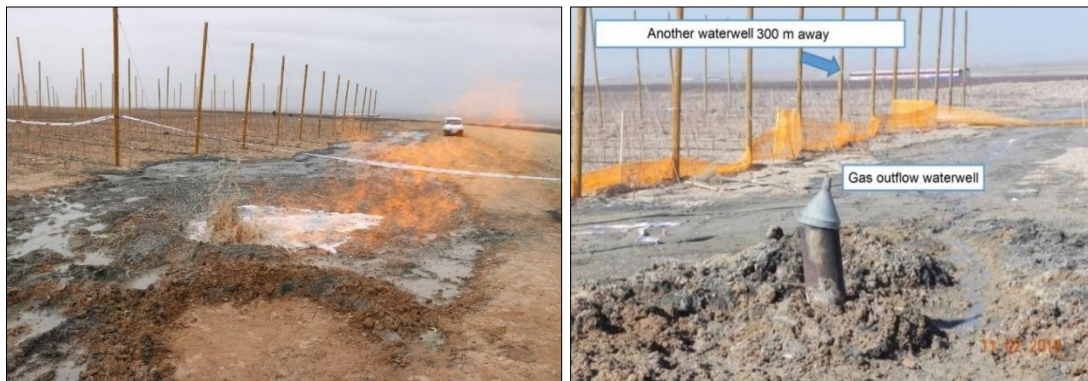
Figure 4. The image of gas outflow in the water well in the Alpağut region (Ulukışla) and the locations of the wells from where the gas and water samples taken.
