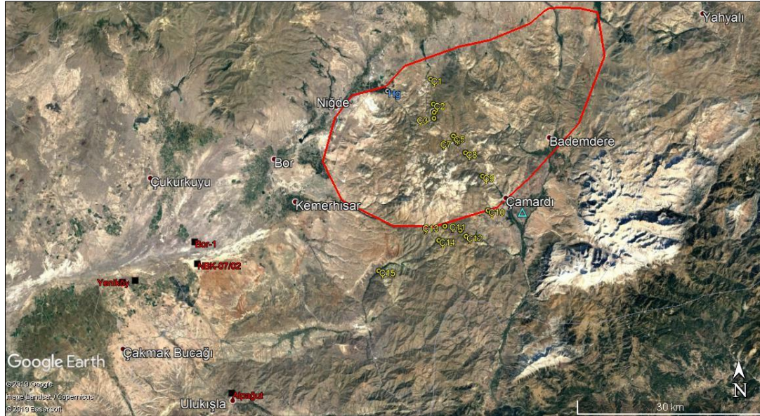
Figure 2. The hydrocarbon shows in the study area and its surroundings. Red polygon: Niğde Massif, yellow circles: the water samples, turquoise triangle: hydrocarbon show indicated by Erentöz and Ternek [47], black squares: shallow and deep wells also indicating hydrocarbon shows in the region, Hg: formerly operated Gümüşler mercury mine.
