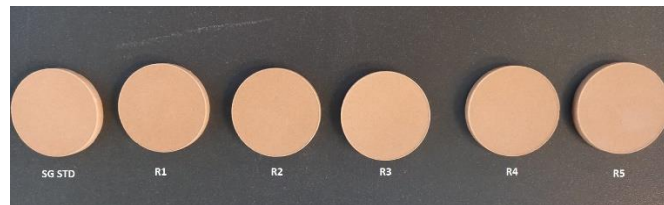
Figure 1 Fired porcelain tile tablets at 1185°C
