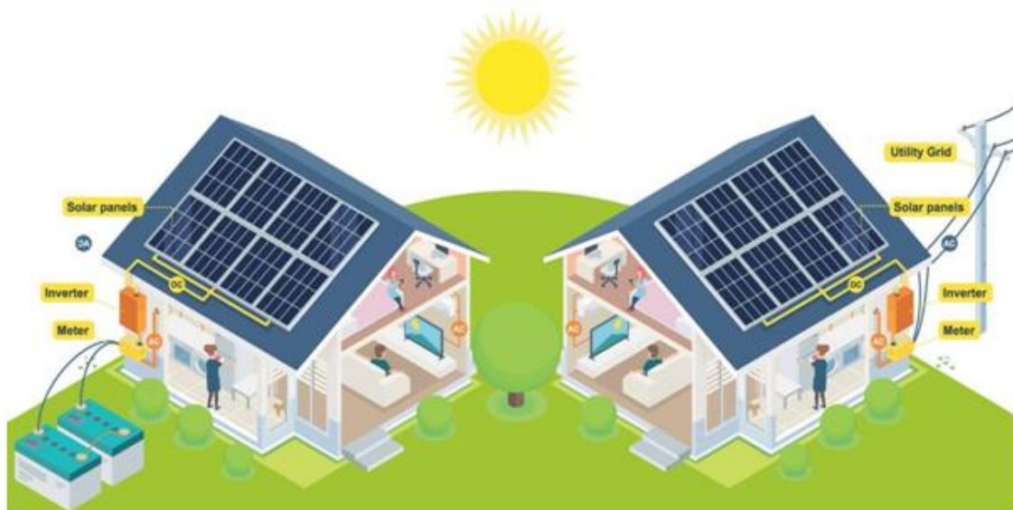
Figure 3. On-grid and Off-grid components [8]
