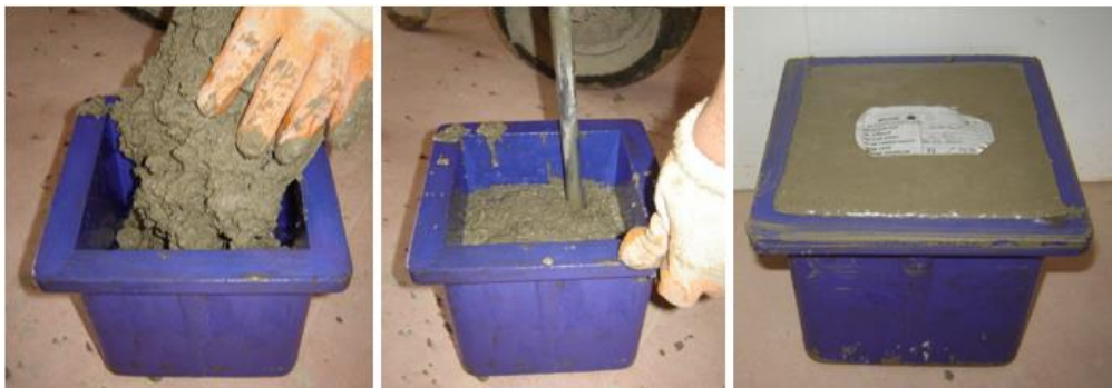
Figure 2. Filling the molds with concrete
