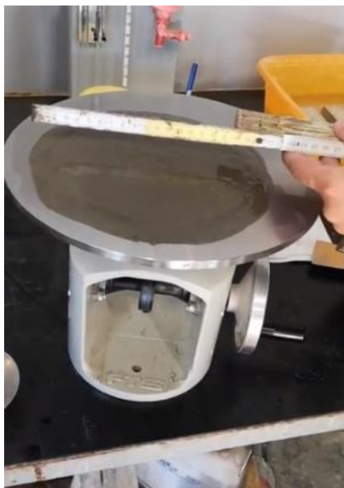
Figure 2. Testing the mortar consistence by flow table
