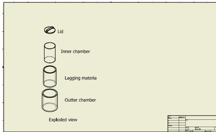
**Figure 2.** Exploded view of the fermentation bin
